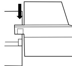
Fill both sides to pocket underside
