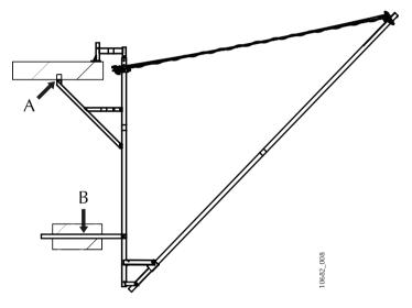
Figure 7. Roof fitting option, anchor in A or B
