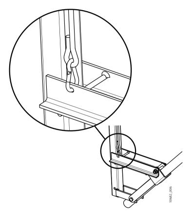
Figure 5. Fitting the control line to the wind lock
