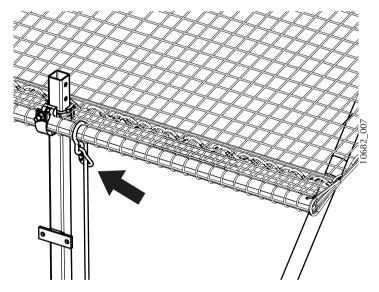
Figure 6. Securing the control line to the safety net fan
