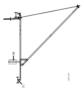
Figure 8. Steel girder fitting option, anchor in B or C
