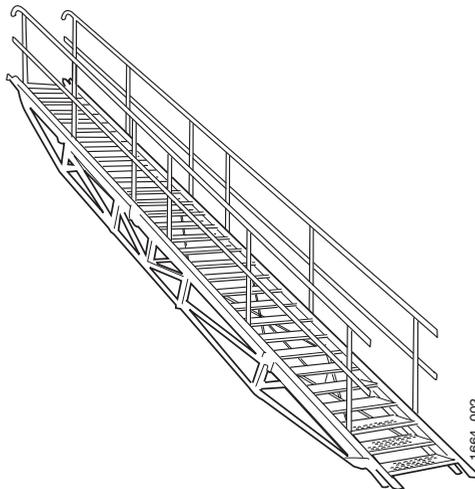
Figure 24. Combibeam in combination with long (coupled) stairways
