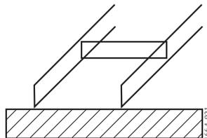
1. Connect the crane to a sling around the upper part of the stairway, put the sling around a step and within the handrails, so that the handrail and stairway are able to open. Make sure the sling is not around the centre of the step, or it may be bent.
