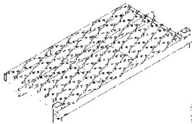
Figure 8. Replacement top step with post sockets
