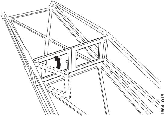
Figure 25. Beam sections with the cross braces downwards
