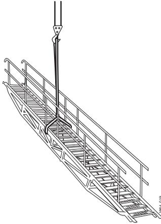
Figure 29. Connecting the crane sling to the stairway and beam
