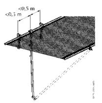
Figure 46. Positioning of the facade attachment
