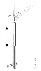
Figure 61. The extension in the safety net fan frame
