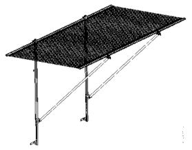
Figure 62. Safety net fan with extension
