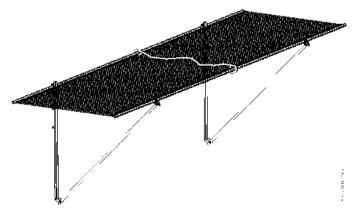
Figure 38. Assembled safety net fan
