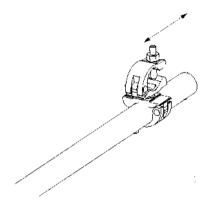
Figure 24. Adjust the double coupler spacing
