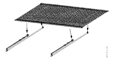
Figure 34. Secure the fan to the frames and tubes
