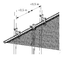
Figure 50. Positioning the scaffold attachment
