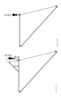
Figure 40. Anchorage loads
