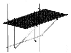
Figure 52. Safety net fan installed on a scaffold with the scaffold attachment
