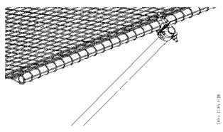
Figure 37. Assemble the outer tube on the raking tube
