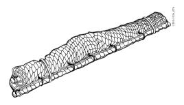
Figure 6. Storage and transport of the safety net fan
