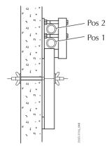
Figure 47. Levels within the facade attachment
