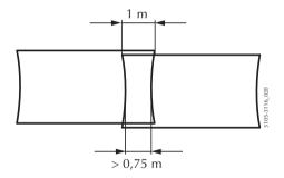
Figure 17. Fall-arrest fan overlap
