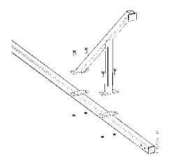
Figure 41. Assembling the knee brace on the frame
