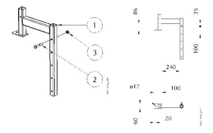
Figure 7. Slab attachment
