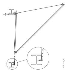
Figure 64. Safety net fan with extension supported on a steel beam
