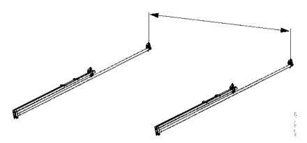
Figure 27. Place the frames with the correct c-c spacing
