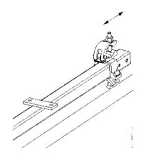
Figure 26. Positioning of square-round coupler
