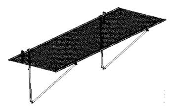
Figure 48. The safety net fan installed within the facade attachment
