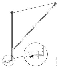
Figure 63. Extension anchored to the slab
