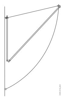
Figure 20. Tying down the safety net fan for high wind
