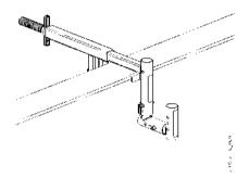
Figure 53. Multi-clamp with elbows installed on a wall top/upstand
