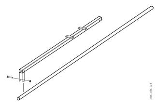
Figure 22. Assembly of frame and brackets
